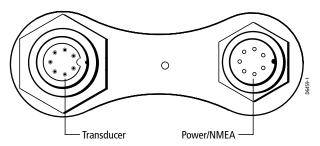
Figure 2-5: DS400/500 Connector Panel
